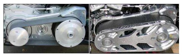
Install front and rear pulley covers. It is suggested that the bolts be loctited.
