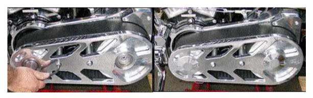
Install buttonhead bolts to secure support to the stand-offs.
