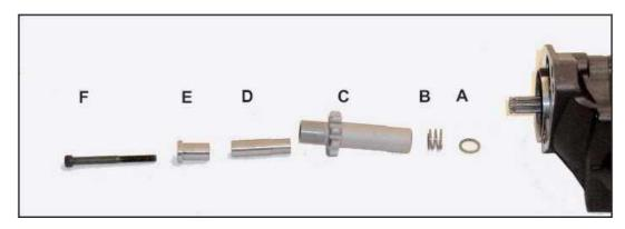
A. Install spring seat on to starter shaft.
