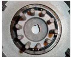
1. Remove stock cage and stock bearings. With grease, coat bearing surfaces of clutch hub and clutch basket.
