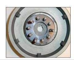
**3.** Place the stock cage retainer (with lip facing out) over nylon shield **4.** Install the 3 springs over studs Pictured right is how cage retainer is installed with lip facing out
