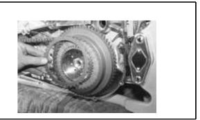
**14.** Install 9 hole pressure plate, use only 6 springs and shoulder bolts. Tighten bolts until they bottom out, this is the correct procedure. The other 3 springs and bolts may or may not be needed depending on how much spring pressure is needed.
