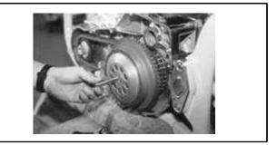
**16.** Install outer primary cover with gasket, tighten all primary cover bolts to HD specifications.
