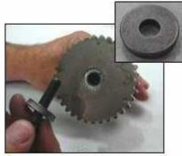
The stock cam bolt and washer must be removed as pictured left and the washer (inset picture) will not be used.
