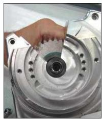
Install the cam end adaptor and special bolt, supplied with kit, and make sure that the slot in the cam end adaptor is at the 7 o'clock position.
