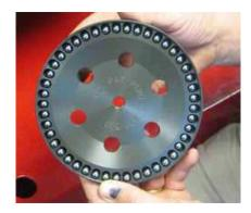
Lock up for Primo belt 390-2007. plate with 42-5/16 " m steel ball bearings.
