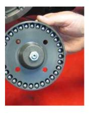
BDL pressure plate with 32 comium steel ball bearings and djustment screw and nut.
