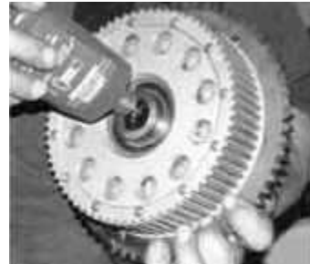
Fig. 6 Use loctite on spline hubs to ensure proper fit on mainshaft
