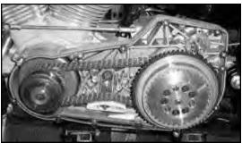
2. Drain primary fluid, and remove outer primary cover and gasket.
