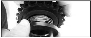
7. Thread carrier body into sprocket, make sure nylatron washer seats fully into the recessed pocket.
