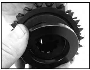
9. Install the rear steel spacer, "steel spacer goes on top off nylatron washer". When assembled steel spacer should sit just below the height of carrier body.
