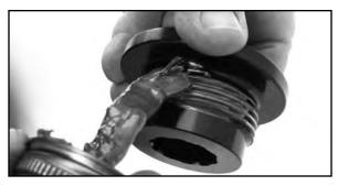
4. Evenly apply a small amount of Anti-Sieze to all of the threads of the compensator sprocket carrier body.
