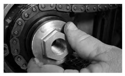
10. Apply RED loctite to threads of the output shaft.
