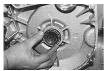
If you are using the stock bearing, then install enclosed seal, flat side facing in.
