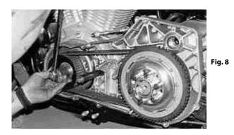
**8.** Apply loctite to and install and tighten to HD specifications, mainshaft hub nut. We supply a special hub nut with seal for all spline shaft models 1990 and later.
