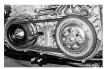
Fig. 11a Finished installation. Be sure to check clearance of outer cover to drive.
