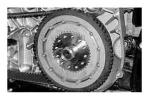
Fig. 9 Install sealed mainshaft nut supplied with 1990-upkits only. For 1986-89 you must use stock hub nut and the seal kit enclosed with kit. For Shovelhead you must use the stock hub nut with seal. Apply loctite to nut before installation.
