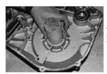
Grease bearing and install seal. It may be easier to use a solid bar to press seal into place. It may be necessary to re-pack bearing and replace seal during yearly maintenance.
