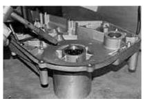
If you are going to remove the stock bearing and use the sealed bearing , then remove primary, remove retaining rings and heat area around bearing for removal.
