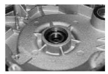
Freeze sealed bearing and re-heat area around bearing housing, the bearingshould fall into place without a problem. Replace retaining ring.
