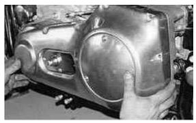
Fig. 12 Install outer primary cover with gasket
