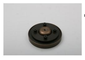
For stock applications, use the black diaphragm spring, Diaphragm collar and the (4) ESB-750 shoulder bolts only, Or for a more stronger force "spring pressure" use the copper colored diaphragm spring instead of the black one. For high performance motorcycles, use both diaphragm springs. For even more spring pressure, place (1) of the (4) AN washers under each head of the shoulder bolts, and on top of the diaphragm spring collar to create even more force "spring pressure" onto clutch pack.
