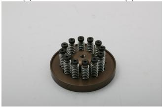
**NOTE:** To achieve the proper spring tension for your application, you can add or subtract springs. Start with six or use any combination 3, 4, 6, 8, 9, 10 or 12 springs. Most high performance applications will only need eight or nine springs.
