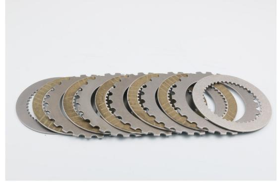
NOTE: All rounded edges on all clutch plates face outward towards pressure plate.
