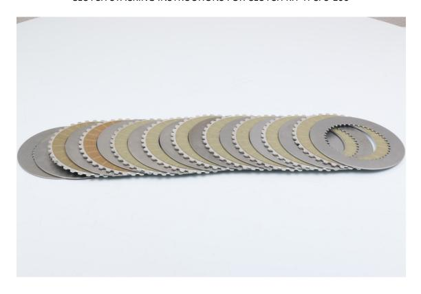
NOTE: All rounded edges on all clutch plates face outward towards pressure plate.
