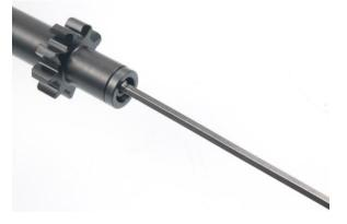
7, Apply a small dab of Anti Seize to the end of the pinion gear that rides in the starter housing bushing.
