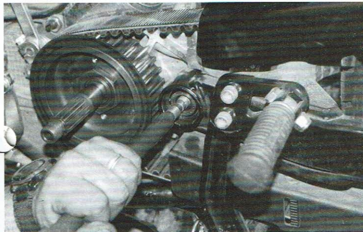
Pict.-3 - Push shaft through by using a blunt drift, so that the swing arm stays intact.
